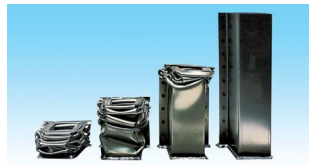
Drop impact test (the middle two products are high-tensile-strength steel materials)
