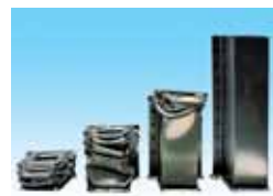
Drop impact test: The high-tensile-strength steel material is the second from the right.
