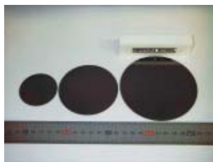
Left to right are shown 2-inch, 3-inch and 4-inch (100mm) single crystal SiC wafers
