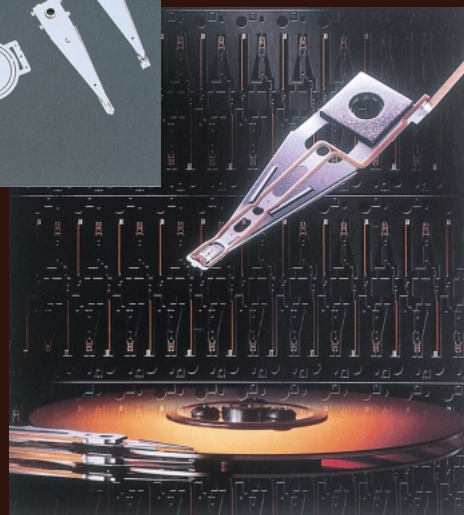
Stainless foil in a hard disk drive
