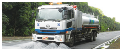
These trucks spray water on the road and empty lots or clean the road within works to restrict the secondary scattering of dust.
