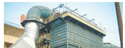
Dust generated in the burning process is collected by two types of dust collectors (electric or with bag filter), depending on the characteristics of the dust (i.e., particle size distribution, emission gas concentration.)
