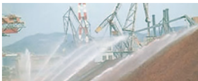
Water and chemical are sprayed on piles of iron ore and coal to restrain the scattering of raw materials.
