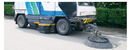
These trucks spray water on the road and empty lots or clean the road within works to restrict the secondary scattering of dust.
