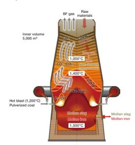
Reduction reaction in blast furnaces
