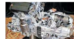
Example of high-efficiency motor using electromagnetic steel sheet
