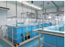
Sea Laboratory (marine environment simulator)
