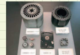
High-efficiency non-oriented electrical steel sheets
