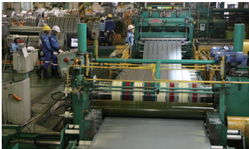
Cutting and processing of base sheets into products with shapes and dimensions conforming to user needs, and just-in-time delivery of finished products (BECC)
