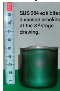
SUS 304 Two-stage drawings (drawing ratio: 2.2)
