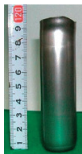
NSSC 304JS Seven-stage drawings (drawing ratio: 4.4)
