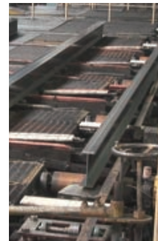
H形鋼 Rolling of H-Shape Beam
