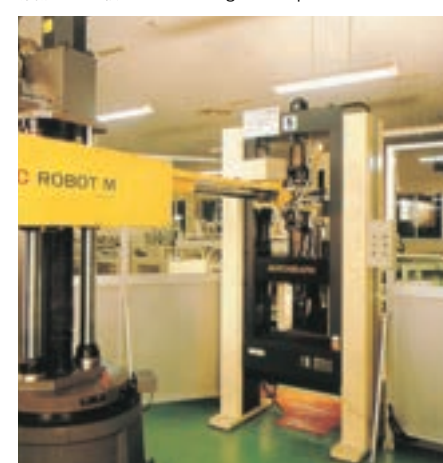
無人試験装置 Full Automatic Tensile Strength Inspection Machine
