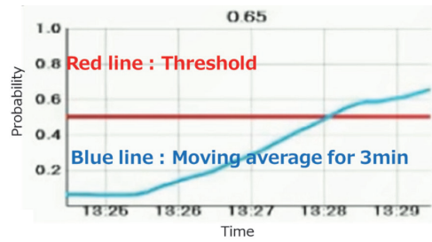
図6 板寄り予兆検知の一例 2) An example of predictive detection of moving coil 2)
