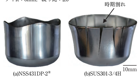
図10 NSS431DP-2 ® 、SUS301-3/4Hの深絞り成形品 Fig.10 Deep drawing parts of NSS431DP-2 ® and SUS301-3/4H.
