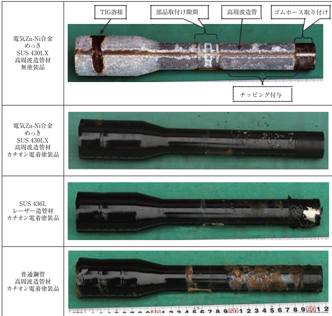
図9 CCT180サイクル後の自動車給油管模擬加工品の腐食状態 Fig.9 Appearance of specimens imitates the fuel pipes after 180 cycles of CCT.
