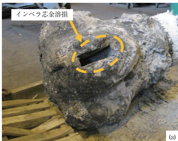
図11 インペラ損耗状況 Fig.11 Appearances of worn out impellers.
