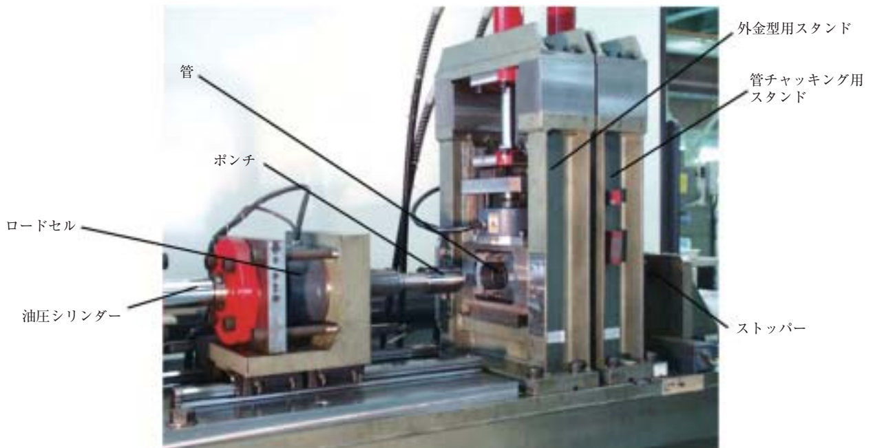
図6 拡管成形試験装置の外観 Fig. 6 Appearance of tube expanding test device.
