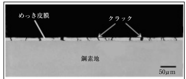
図15 円筒絞り加工側壁部の断面組織 (ZAM60) Fig.15 Cross-sectional structure at the wall of drawn cup (ZAM60).
