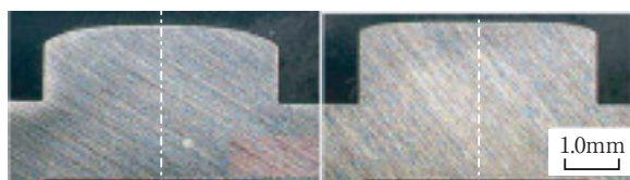
(a) Steel A焼鈍材 (b) Steel B-10%調質圧延材
