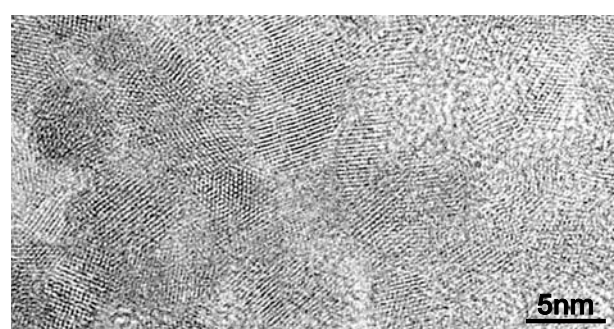
Fig.14 High resolution TEM micrograph of corrosion products formed on Zn-6Al-3Mg coated steel sheet at the position 3 in the bright field image of Fig.13.
