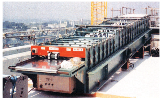
図10 折板ロール成形機 Fig.10 The conventional folded-plate forming machine used.
