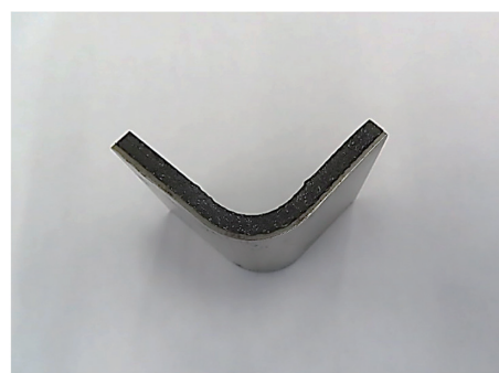
Fig. 2 Appearance of CFRP and steel composite after press forming
