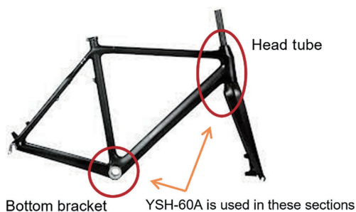
Fig. 6 Example of using YSH-60A fiber to stiffen ultralight road bicycle frames
