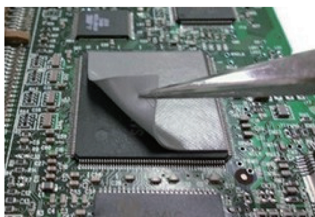
Fig. 10 High thermal conductive silicone sheet with high thermal conductive pitch-based carbon fiber
