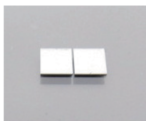
(a) Chip mounting image Mounted in parallel at 100μm intervals
