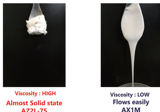
Fig. 10 Change in resin flowability with the addition of fine spherical alumina filler AX1M
