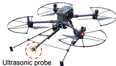
Fig. 3 Drone equipped with ultrasonic thickness gauge
