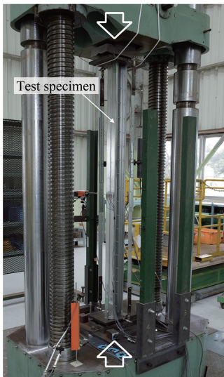
(a) Long column compression test
