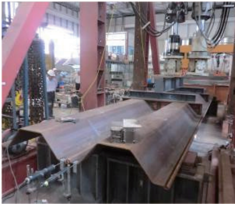
Fig. 3 Outline of flexural test of HAT-type steel sheet pile wall
