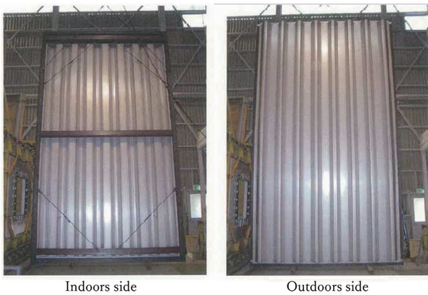
Indoors side Outdoors side Fig. 6 Specimen of wind pressure resistance test
