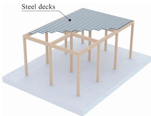
Fig. 3 Structure of Timber NBR construction method™
