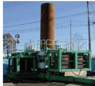
Photo 4 Pile rotary machine 6)
