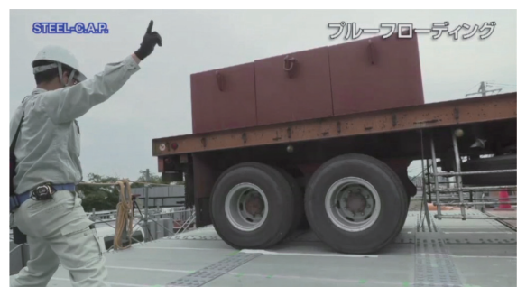
Fig. 5 Proof-loading test using the mock-up test specimen
