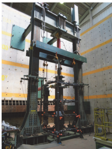
Photo 4 Overview of full-scale structural test of “SOKKETSU KANBEE™”
