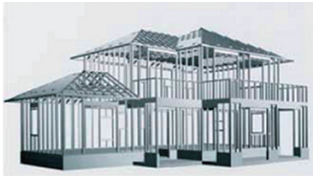
Fig. 6 Steel framed house
