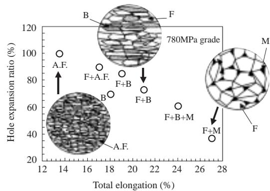
Fig. 10 Relation between total elongation and hole expansion ratio of 780MPa as-hot-rolled steels, and their microstructural feature
