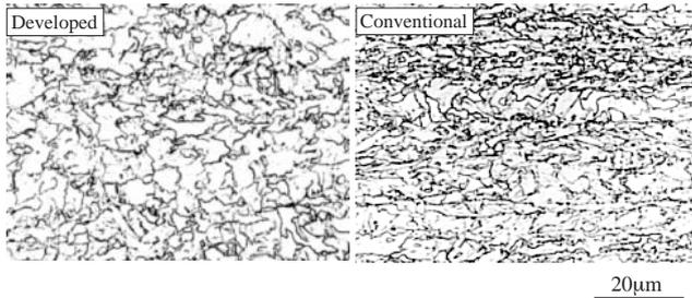
Fig. 12 Microstructures of developed and conventional 780MPa grade steels
