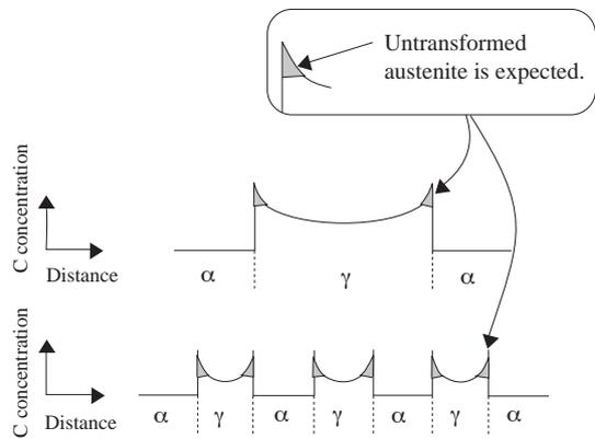
**Fig. 4** Carbon concentration profiles in ferrite and austenite during the formation of ferrite
