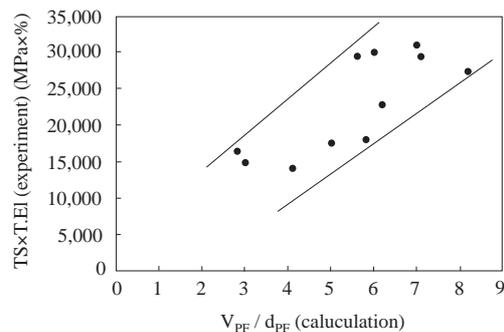
**Fig. 5** Effect of the ratio between volume fraction and grain size of polygonal ferrite ( $V_{PF}/d_{PF}$ ) on  $TS \times T.El$  of as-hot-rolled low-alloy TRIP steels
