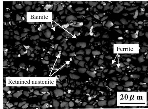
**Fig. 3** A typical optical microstructure of as-hot-rolled low-alloy TRIP steel (special etching<sup>4)</sup>)
