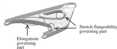
Fig. 9 Appearance and required forming properties of a lower arm
