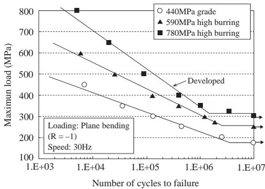
Fig. 13 Fatigue property of developed 780MPa grade high burring steel (plane bending fatigue test)
