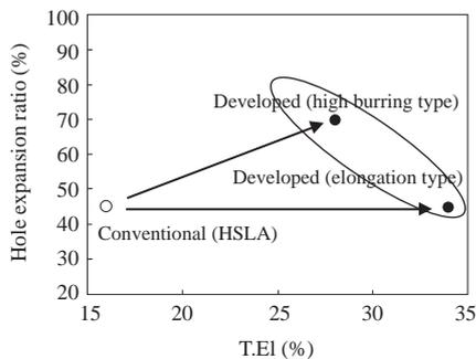
**Fig. 6 Elongation-hole expansion ratio combination of developed as-hot-rolled low-alloy TRIP steels**
