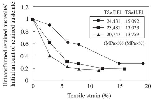
**Fig. 2** Change in volume fraction of retained austenite as a function of tensile strain and the effect of stability of retained austenite on the strength-elongation combinations
