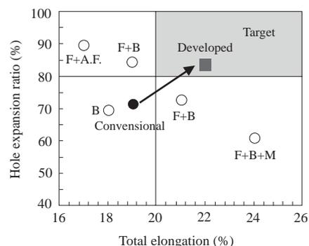
Fig. 11 Combination between total elongation and hole expansion ratio of developed 780MPa steel
