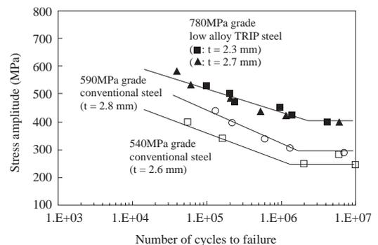
**Fig. 8 Fatigue property of 780MPa grade as-hot-rolled low-alloy TRIP steels (plane bending fatigue test)**
