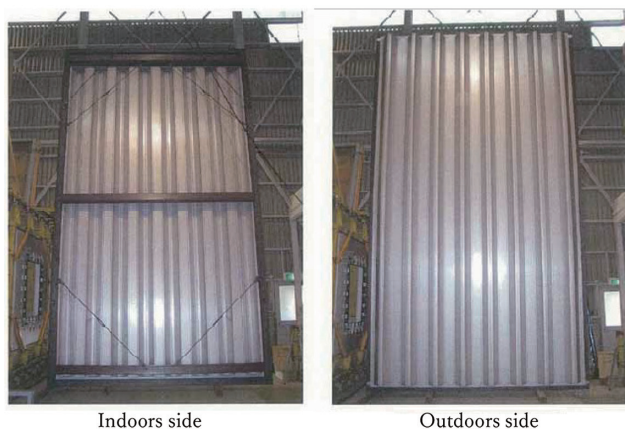
図6 耐風圧性能試験の試験体 Specimen of wind pressure resistance test
