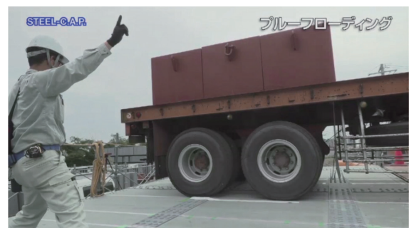
図 5 載荷試験状況 Proof-loading test using the mock-up test specimen
