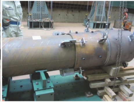
(b) Joint of support column and joint
